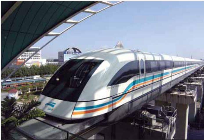
The Shanghai maglev, shown here at the Long Yang Road Station, is the only operational maglev in the world. Its maximum speed is 311 mph.
