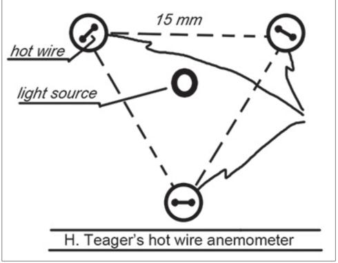
Air passing around a wire cools it, changing its electrical resistance, which can be detected by the same attached wire which is electrically heating it, measuring the amount of air flow passed the apparatus.
