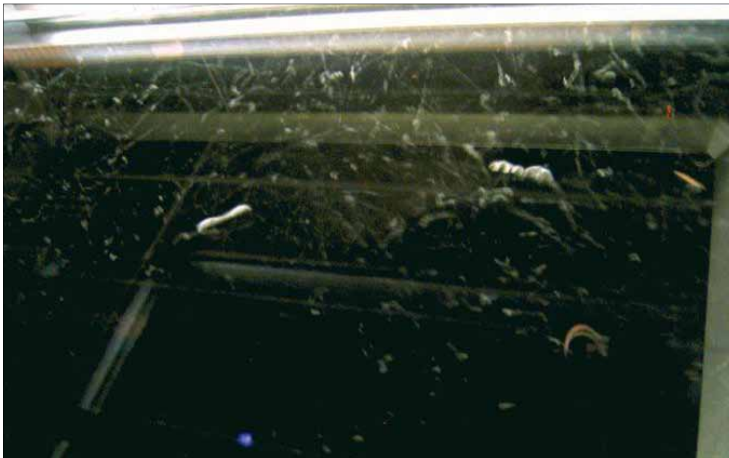
Tracks of ionizing radiation from cosmic rays, in a cloud chamber. The thick, short tracks are alpha particles; the long, thin ones are beta particles. C.T.R. Wilson perfected the first cloud chamber in 1911.
