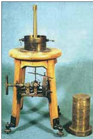
A sample of pitchblende, the ore containing uranium. The Curie electrometer, invented by Pierre and his brother Jacques.
