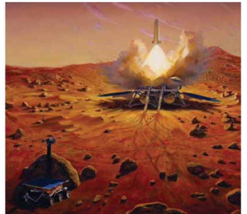
Before men are sent to Mars, in 2024, an international robotic mission will be deployed to return samples of rock and soil to be intensively examined in laboratories on Earth. In this artist's representation, an ascent vehicle is taking off from the Martian surface, to deliver its previous cargo. The rover, which collected the samples and delivered them to the vehicle, takes shelter behind a rock. JPL/NASA
