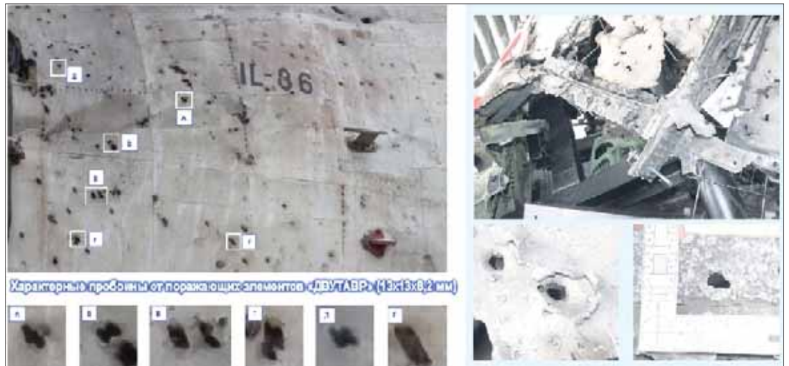
Left, the signature bowtie-shaped holes left by the 9N314M warhead's “double-T” shrapnel. MH17 (right) lacks similar damage. Photos: left, Almaz-Antey; right, Dutch Safety Board
